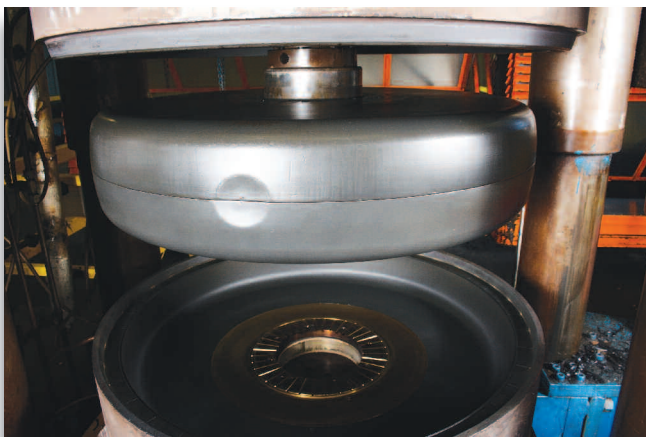
CMT mold ready for loading and envelope curing.
