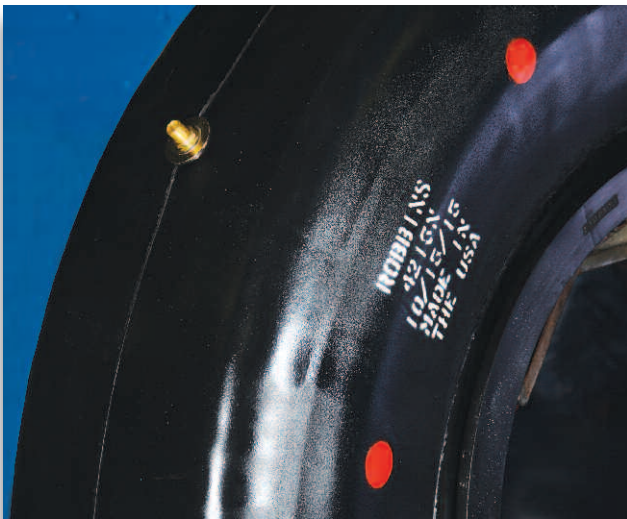
Compression Molding Technology (CMT) from Robbins uses proprietary rubber compounds that are placed into a mold for curing, which eliminates splicing the envelope, increasing production life.
